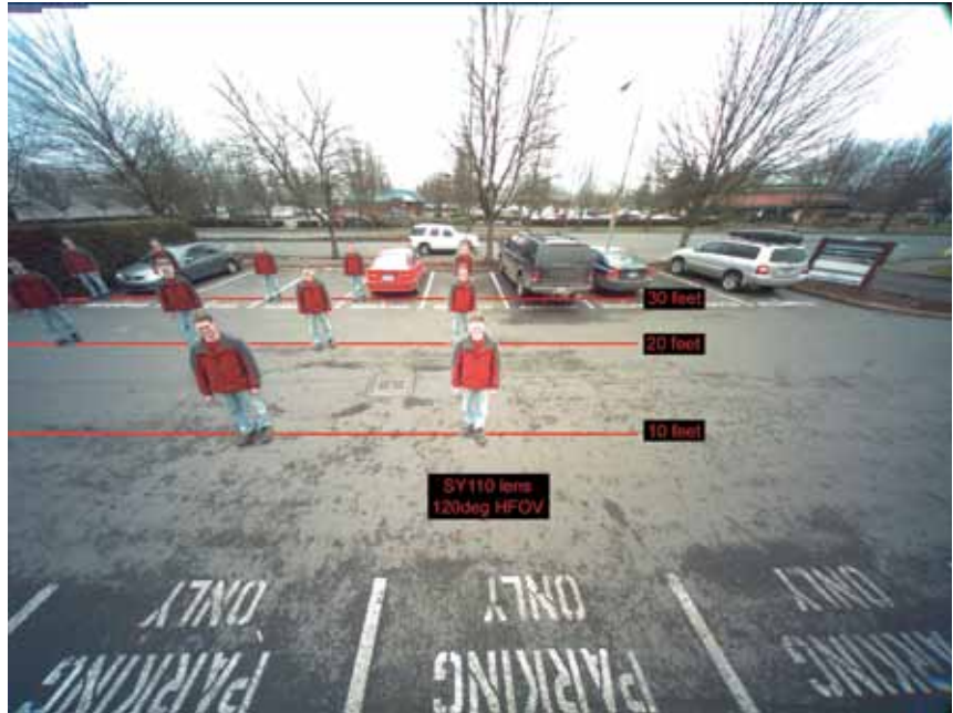
Figure 3 These targets are in a 10 x 10 feet grid. At 20 feet from the camera using Theia's lens with 120-degree field of view, the horizontal field of view (HFOV) is 60 feet. Targets at the edge of the image are twice as far from the camera but can be seen as clearly as those in the center of the image along the same plane.
