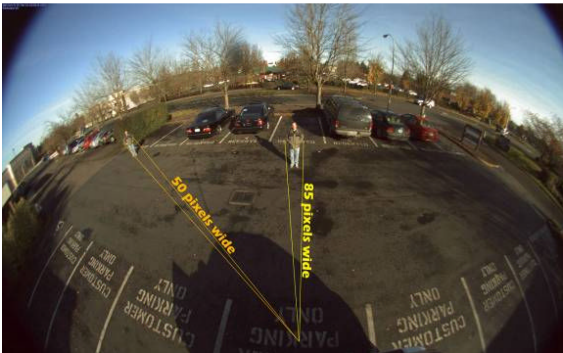
Distortion reduces the object width the further it is from the image center.
